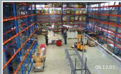
8 DECEMBER 2005: TOMRA PRODUCTION FACILITY, LIER, NORWAY. Production of TOMRA's reverse vending machines is in full swing. (Above) Pictured here is the assembly area for the heart of the RVM, the recognition unit. (Right) An area previously used for storage now is being made ready as an assembly line for mounting the upper recognition units to the bottom collection cabinets.
