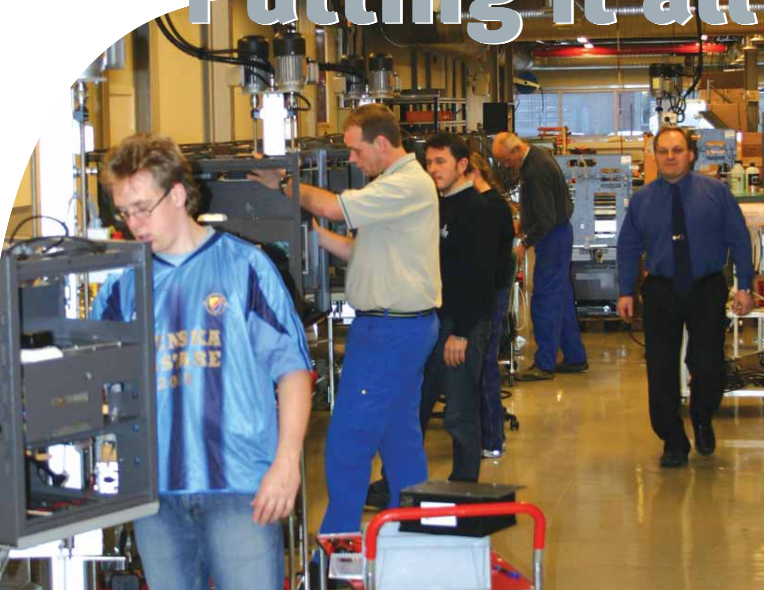
8 DECEMBER 2005: TOMRA PRODUCTION FACILITY, LIER, NORWAY. Production of TOMRA's reverse vending machines is in full swing. (Above) Pictured here is the assembly area for the heart of the RVM, the recognition unit. (Right) An area previously used for storage now is being made ready as an assembly line for mounting the upper recognition units to the bottom collection cabinets.
