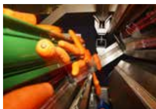
The HALO's NIR optical sensors sorts carrot product for shipment.
