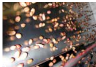
The Nimbus's lasers and BSI module inspects peanuts during free-fall.
