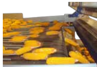
The ZEA's NIR optical sensors sort seed corn.
