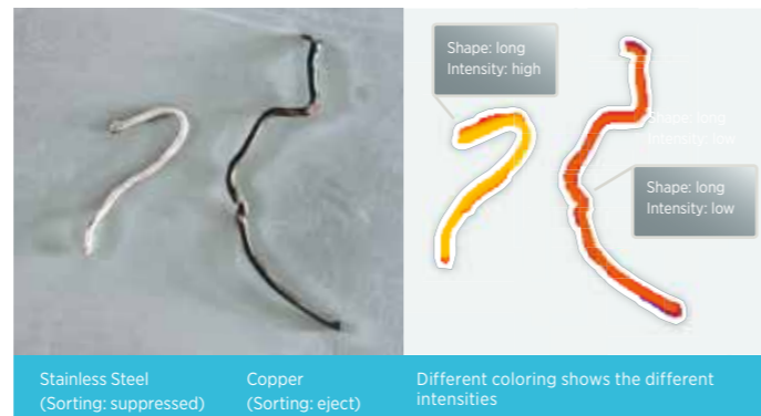
New DEEP DATA technology increases sorting performance and stability
