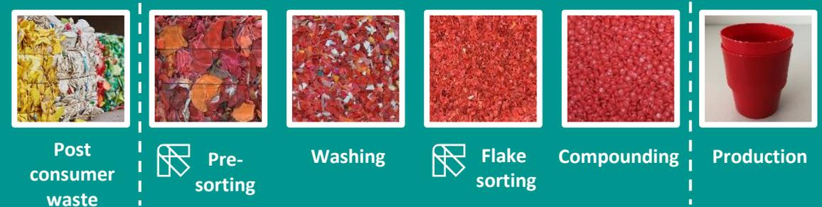
The demo plant covers the process from post consumer waste to production of recycled polymers.
